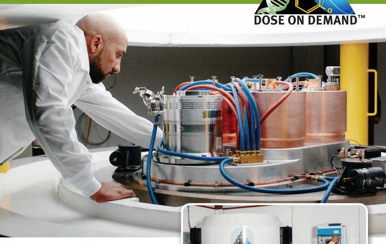
The BG-75 Biomarker Generator integrates a compact mini-cyclotron, kit based micro-chemistry, and automated quality control, simplifying in-house production of <sup>18</sup>F-FDG and advanced biomarkers.
