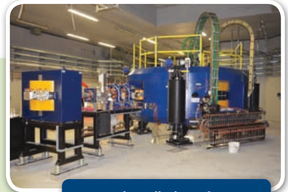
Installation of Best 70 MeV Cyclotron at Italian National Laboratories (INFN) Legnaro, Italy
